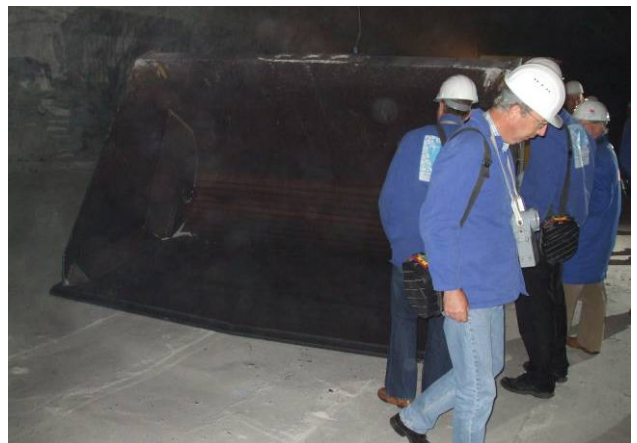
Modern machinery for removing the freshly blasted rock. Each bucket full of the loader weighs approximately 12 tons. These loading shovels are used to move rock from the mine face to the conveyors and crushers that transport ore around the mine or to the mine shaft for lifting to the surface.
