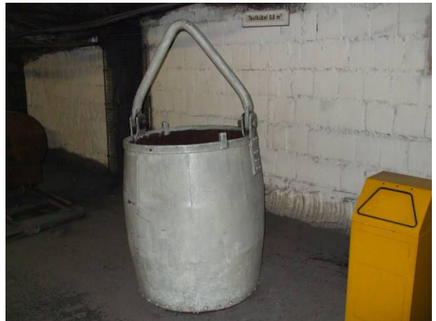
The original bucket used to begin mining in 1899. The bucket capacity is 0.8\text{m}^3 , and would have been lowered into the mine shaft with one or two workers.
