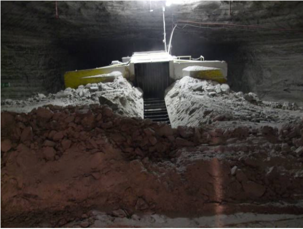
Crusher and conveyor for moving ore around the mine
