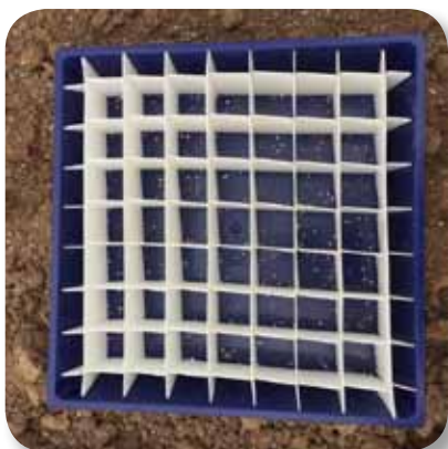
Figure 6:- Examine the fertiliser granule distribution in the trays and then take fertiliser from trays and weight
