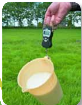
Figure 11:- For twin disc machines multiply fertilizer weight by 2 to get application rate.
